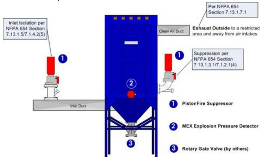
**5) Suppressed Dust Collector with Chemical Inlet and Outlet Isolation**
