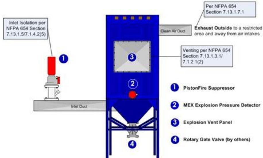
**4) Suppressed Dust Collector with Chemical Inlet Isolation**
