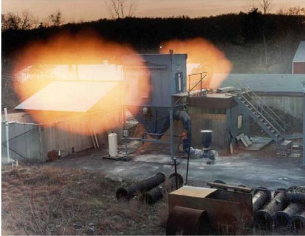
Picture 2 – Vented and isolated explosion
