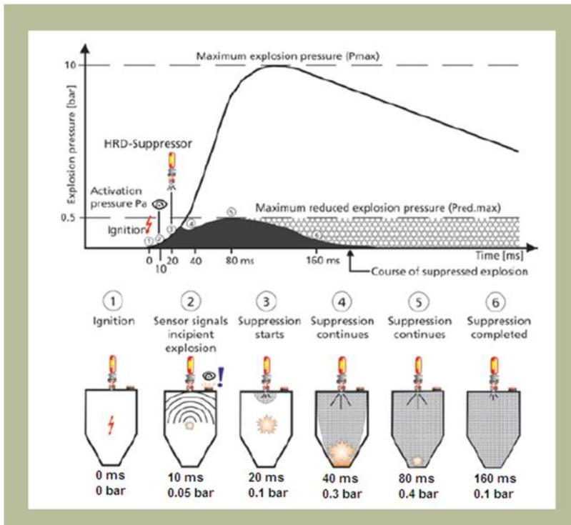
Figure 1 – Steps in explosion suppression<sup>9</sup>
