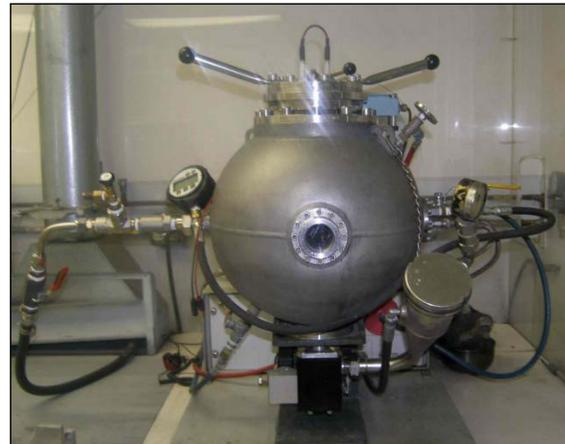
Figure 1: 20 L vessel used in dust deflagration testing.
