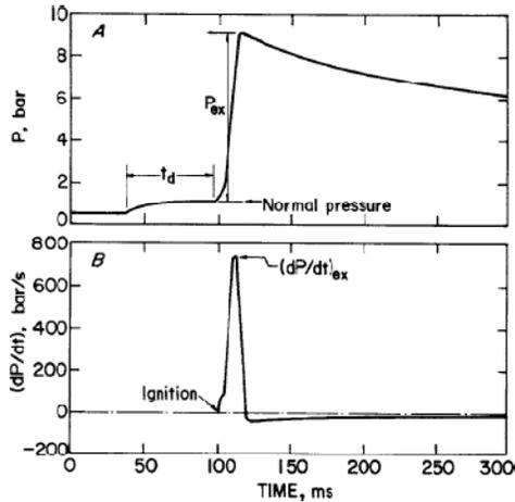
**Figure 2: Typical graph showing  $P_{ex}$  and  $dP/dT_{ex}$  for a dust deflagration.**
