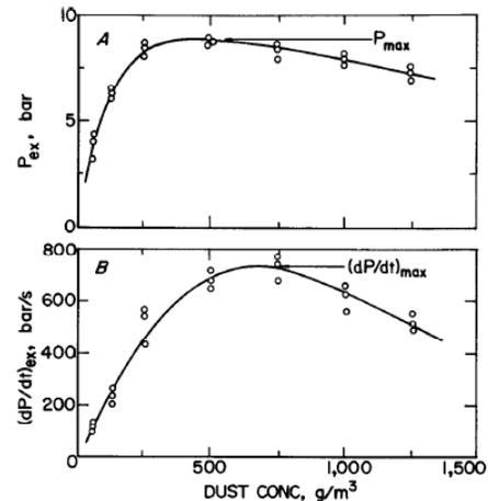
**Figure 3:  $P_{ex}$  and  $dP/dT_{ex}$  data as a function of dust concentration for determining the optimum deflagration concentration and equivalent  $P_{max}$  and  $R_{max}$ .**<sup>1</sup>
